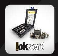
Loksert® key-locking thread inserts are used to quickly repair stripped, damaged or worn threads with new stronger threads, or for use in original equipment. Lokserts are easy to install and remove. No special drills, taps or prewinder tools are required. Their solid, one-piece construction provides a high degree of pullout strength and the keys provide a positive mechanical lock against rotation
