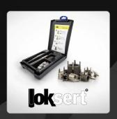
Loksert® key-locking thread inserts are used to quickly repair stripped, damaged or worn threads with new stronger threads, or for use in original equipment. Lokserts are easy to install and remove. No special drills, taps or prewinder tools are required. Their solid, one-piece construction provides a high degree of pullout strength and the keys provide a positive mechanical lock against rotation.
