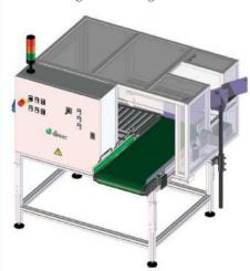
the conveyor belt movements for the positioning of the empty boxes at loading position, the forward movement of the roller outgoing and backward of the same roller on the filling position to receive the empty boxes. The operator's tasks are limited to adjust and po-
