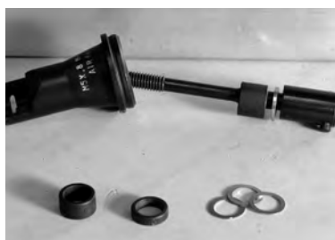
Front end assembly with longest spacer to suit 1.0D insert and shim washer.
