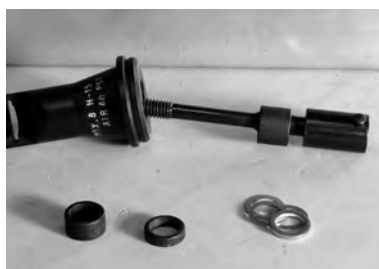
Front end assembly with longest spacer to suit 1.0D insert.
