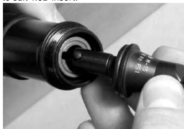
Front end assembly with longest spacer to suit 1.0D insert.
