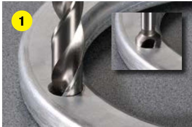
Drill with a standard tap drill and countersink with a standard 82°-100° countersink tool; see tables for correct dimensions.
