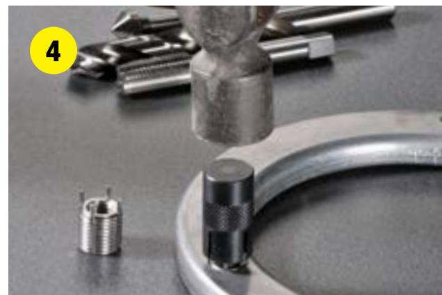
Drive keys down with several hammer taps on the specified installation tool.
