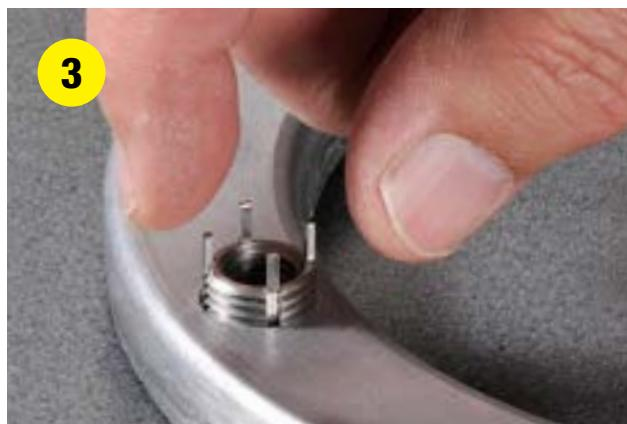
Screw in the insert until it is 0.25-0.70 mm (0.010-0.030 inch) below the surface. Insert keys locate the Loksert at the correct depth.
