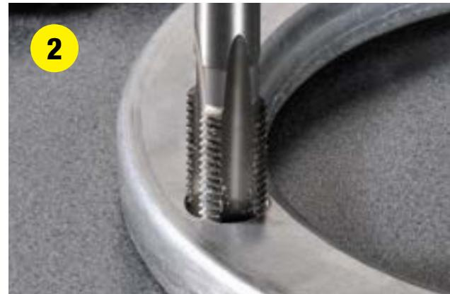
Tap new threads with a standard tap; see tables for correct dimensions.
